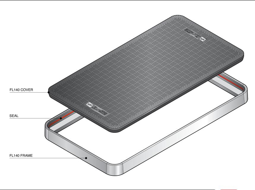
1400mm x 700mm flat sealed composite cover and aluminium frame.
