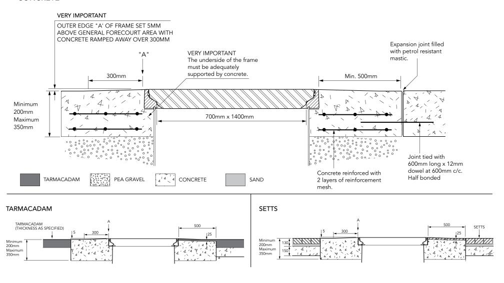
1400mm x 700mm flat sealed composite cover and aluminium frame.
