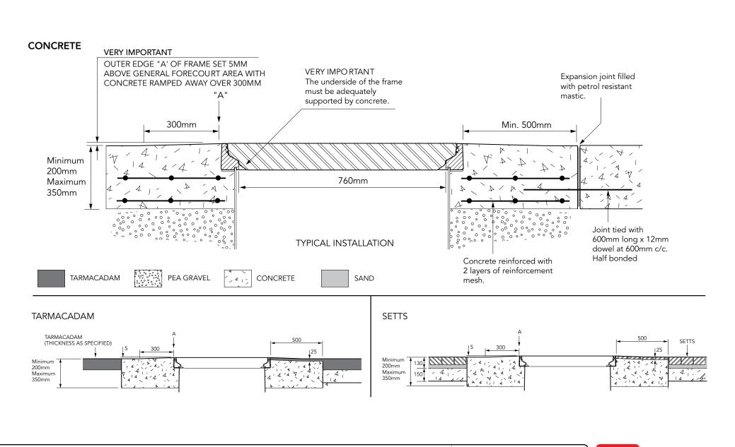
760mm x 760mm flat sealed composite cover with an aluminium frame.
