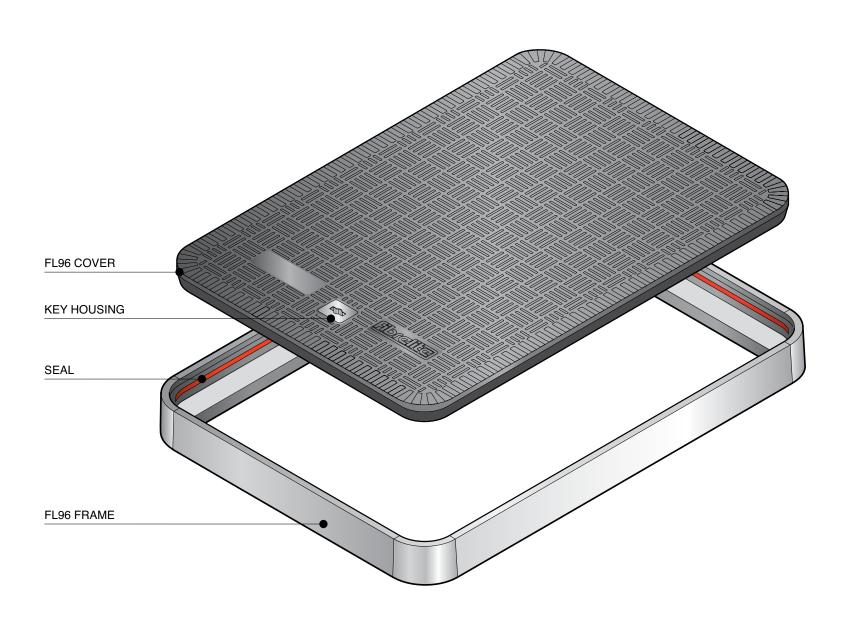
$900 \times 600 \text{mm}$  flat sealed composite cover with an aluminium frame.
