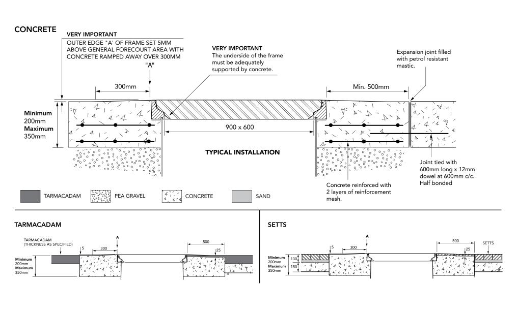
900 x 600mm flat sealed composite cover with an aluminium frame.
