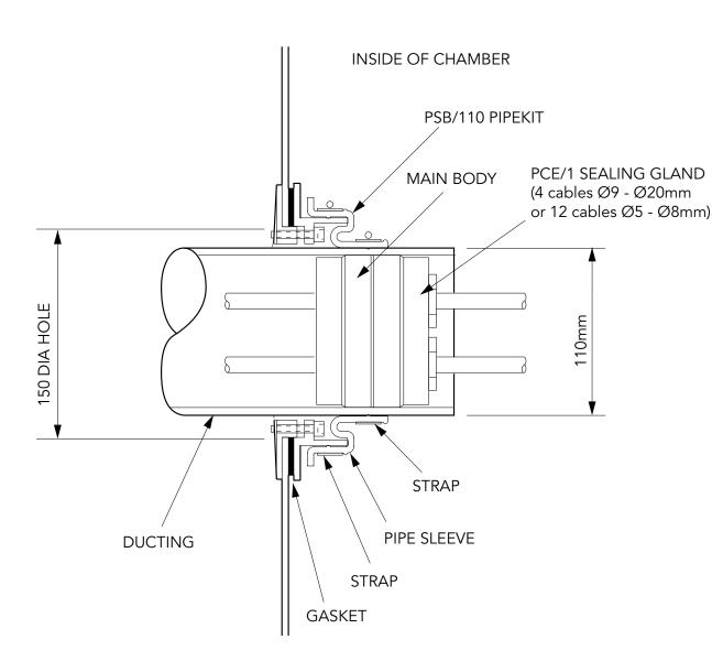
The PCE/1 sealing body is capable of sealing to ducts with an internal diameter ranging from 97 to 110mm.
