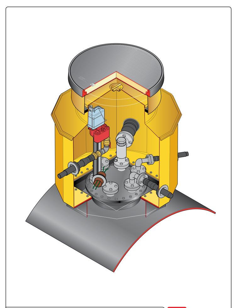
1.5m diameter 12 sided sump with solid base and manway lid adaptor, corbel, adjustable height skirt, internal lid, and round 1020mm flat sealed cover and frame
